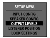
When MC-1 input and output levels are set properly, the entire system will be calibrated to play films at the level intended by the director. Setting the output levels is easy with a Sound Pressure Level (SPL) meter. Using the MC-1's internally generated calibration signal, adjust the level of each output to the same relative level (75dB "C" weighting).
